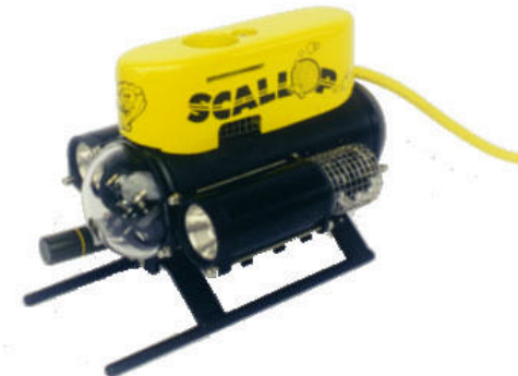
Scallop Outfitted with a GM Tube Radiation Sensors
